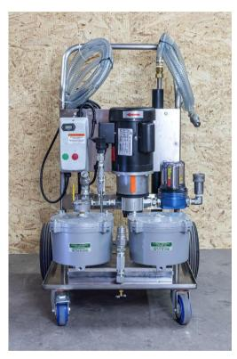
The Micron Filtration System is a multi-purpose fluid cleaning and transfer rig, which is available in a variety of styles and sizes.
