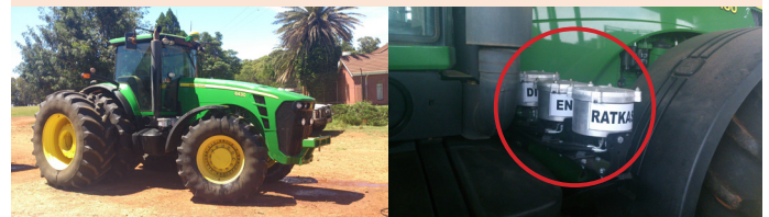
John Deere 8430 New addition to the fleet with KLEENOIL Filtration units installed to the Fuel, Engine and Gearbox before the machine was taken into service.
